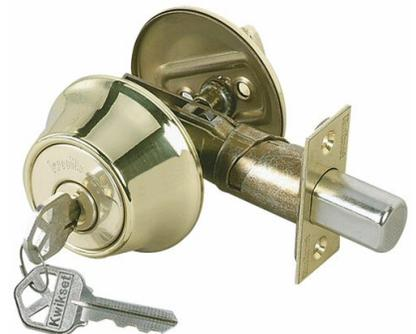
A double cylinder deadbolt lock is key operated from both the inside and outside. It should be used on doors where there is breakable glass in the door or within 40" of the locking mechanism. This makes it impossible for the burglar to break the glass and reach inside to unlock the door.
